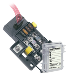
SafetyHub 100 Fuse Block —Holds 3 MIDI® or AMI® and 4 ATO® or ATC® Fuses Vmxo Maximum Voltage: 12V DC Imxo Maximum Amperage per block: 300A DC MIDI® or AMI® Fuse Block— Imxo Maximum Amperage per circuit: 200A DC ATO® or ATC® Fuse Block— Imxo Maximum Amperage per circuit: 30A DC Imxo Maximum Amperage per block: 50A DC
