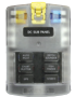
ST Blade Fuse Block (6 and 12 Circuit Models Available)—Uses ATO® or ATC® Fuses Vmxo Maximum Voltage: 32V DC Imxo Maximum Amperage per circuit: 30A DC Imxo Maximum Amperage per block: 100A DC
