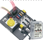
SafetyHub 250 Fuse Block with Remote Battery Switch —Holds 3 MIDI® or AMI® and 4 ATO® or ATC® Fuses Vmxo Maximum Voltage: 12V DC Imxo Maximum Amperage: 240A DC MIDI® or AMI® Fuse Block— Imxo Maximum Amperage per circuit: 200A DC ATO® or ATC® Fuse Block— Imxo Maximum Amperage per circuit: 20A DC Imxo Maximum Amperage per block: 50A DC
